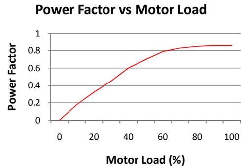
Graph 6. Illustration of Power Factor vs Motor Load
