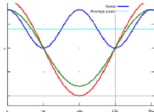
Graph 4. Illustration of Voltage, Current and instantaneous Power Waveforms when PF=1
