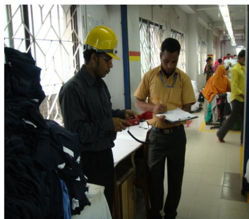
**Picture 3. Ventilation air flow rate test by GTZ Energy Audit team**
