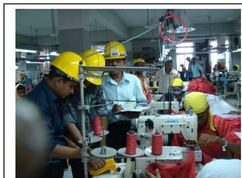
**Picture 4. Sewing motor “No-Load” test by GTZ Energy Audit team**
