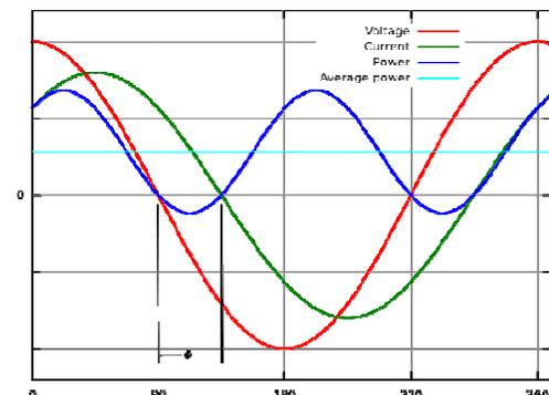
Graph 5. Illustration of Voltage, Current and instantaneous Power Waveforms when PF=0.7.
